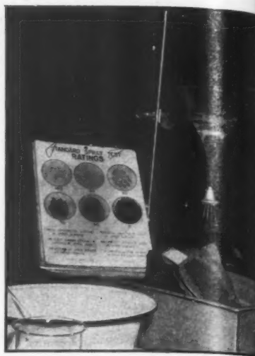
Rainstorm in a pan. In this test Army fabrics are rated according to their water-repellency. Effect of laundering and dry cleaning is carefully gaged.
